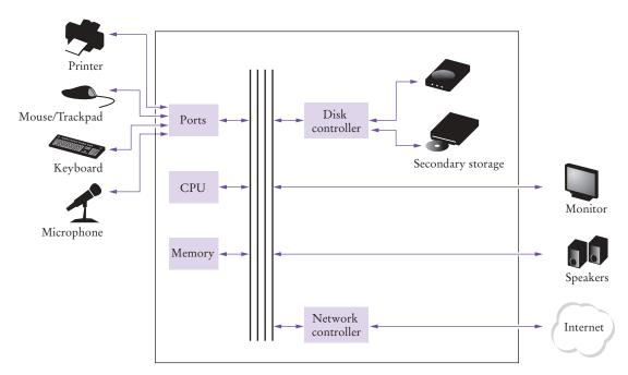
Figure 3 Schematic Design of a Personal Computer
