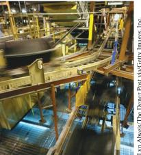
The Denver airport originally had a fully automatic system for moving luggage, replacing human operators with robotic carts. Unfortunately, the system never worked and was dismantled
