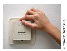
Although a thermostat is usually white, you can think of it as a "black box". The input is the desired temperature, and the output is a signal to the heater or air conditioner.
